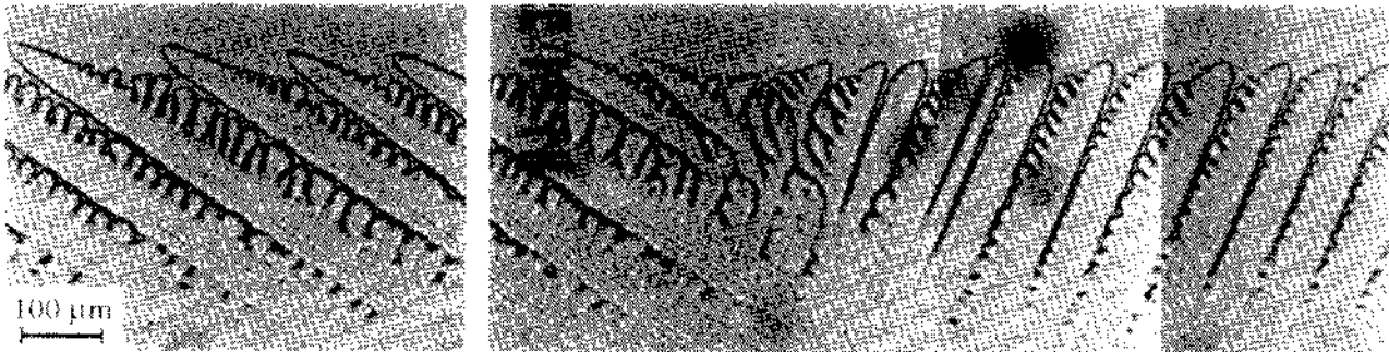
FIG. 25. Competition between two tilted dendritic states in a crystal close to the degenerate orientation (same crystal as in Fig. 4). V = 32 \mu\text{m s}^{-1} ( \approx 17V_{CS} ). Note the dynamic wall between two domains occupied by the [100] ( \phi \approx 22^\circ to the right) and the [010] dendritic states ( \phi \approx 54^\circ to the left), respectively.
