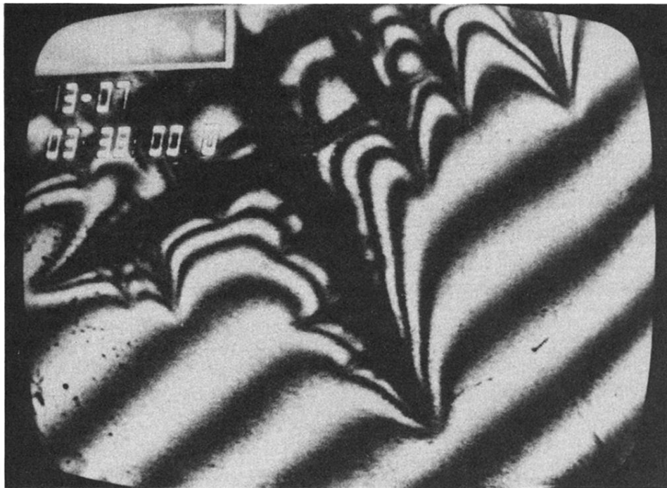
FIG. 5. Interferogram of a growing dendrite with side branches (photographed from the screen).
